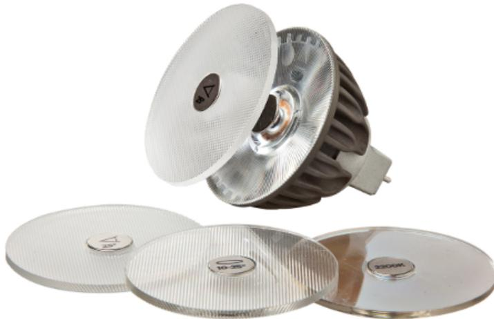
Many filters give various shapes of beams and shades of white. For instance, one filter would render a "warmer" white and another would project a square beam. A magnet sticks the filters at the center of the spot at will. They are 2mm thick only.
